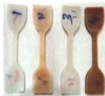
Figure 2. Samples prepared for tensile testing.
